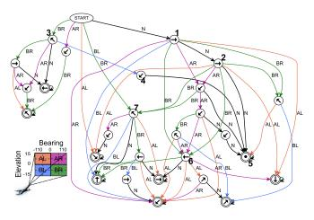
Fig. 3. A subgraph of the policy graph for the 3-D continuous-state POMDP model with EO/IR. Each node is labeled with START, an arrow, or a dot. START indicates the start node. An arrow indicates the directions of vertical acceleration and turn. A dot indicates zero acceleration and turn. Doubly-circled nodes represent initial policies. Each edge is color-coded and labeled with BL (below-left), BR (below-right), AL (above-left), AR (above-right), or N (no detection).
