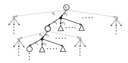
Fig. 4. The belief tree for an SD POMDP. The part in black indicates a policy that makes use of simple sub-policies, each represented as a " $\triangle$ ".
