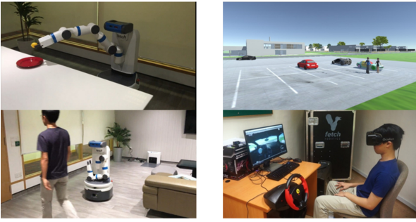
Figure 1. Experiment Task Domains: (Left) Household tasks with the Fetch Research Robot picking and placing objects (top left) and indoor navigation (bottom left) (Right) Autonomous Driving tasks in the Virtual Reality simulation system. Tasks included parking and various navigation scenarios.
